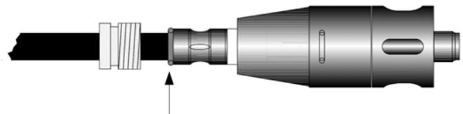
8) Set up the o-ring: no mesh from the shield should be visible. Screw the white thread nut on to the connector housing.
